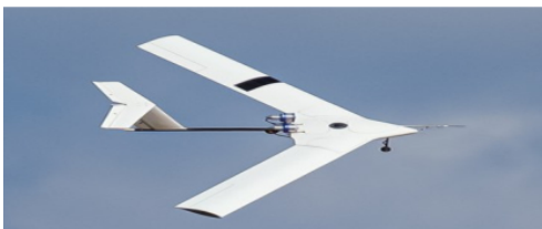
Fig 1: Modified 1/3 scale X56A with 35deg swept wing.
