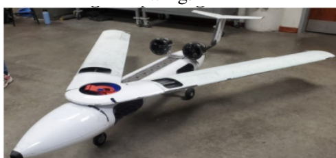
Fig 3: New flight test model allowing variable wing sweep.
